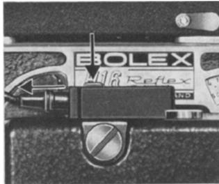
1. Lift the clamp and remove the light-tight cover plate from the camera.
