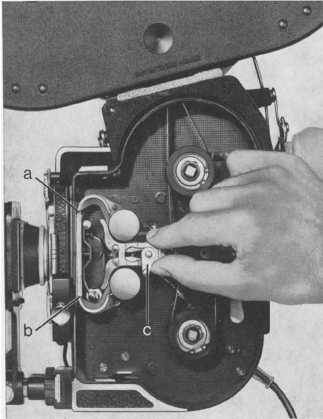
4. Open the pressure plate of the gate.
