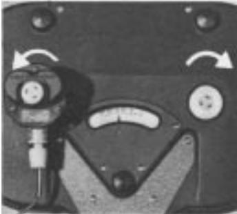
11. Replace the magazine and camera lids and lock them carefully in place.
