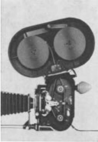
7. Close the loop formers and then proceed with the automatic loading as described in the instruction manual for the camera. Allow about 2 ft of film to run through the lower sprocket.
