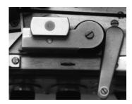
The lever should be pushed all of the way in for forward tape motion.
