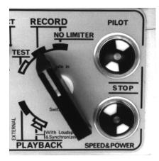
When the main function switch is pointing to the **nine o'clock** position, the Nagra is OFF.
