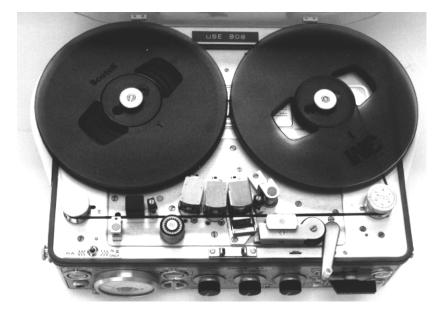
If your Nagra is equipped with a playback shield, make sure that the tape is threaded between the shield and the head, then close the shield over the tape.
