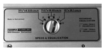
Located between the tape reels, this switch controls the tape speed and bias type. The normal tape speed in our industry is 7 1/2 inches per second.
