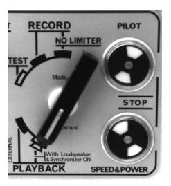
There are two **PLAYBACK** positions on the Nagra. The first PLAYBACK mode is used for non-sync playback in the headphones or line out. The internal loudspeaker does not function in this mode. The **internal resolver does not function** is this mode. This playback mode is used for private quick checks of the audio by the operator, or for locating cue points for playback.
