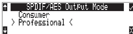
The format for the AES3id output is selectable between professional AES and SPDIF. In either case the SCMS bit is not set.
