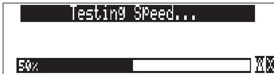
CF cards vary widely in their read and write throughput. Later generation “24x” and greater CF cards can reliably read and write multi-track, high sample rate audio. The 702 includes a drive speed test to measure the throughput speed of CF medium.
