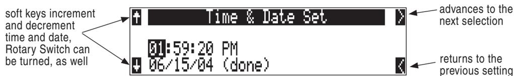
Once set, the time and date clock will be kept while the removable rechargeable battery is attached. If it is removed the internal AA NiMH time code battery maintains the time-of-day and date for 20 days, or more.
