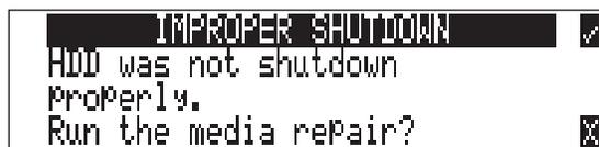
While it is typically safe to disregard this message and hit the soft button X, it is best practice to properly remove the 702 from a Macintosh by dragging the volume to the trash or by using the front panel shortcut ⌘-e.
