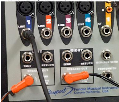
Connect the two speaker wires to the SPEAKER OUTs on the front of the Fender. The other end of the speaker wires should be plugged into the front of each speaker itself, if you have not already done so.
