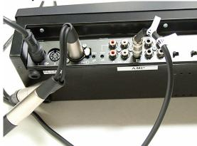
On the back of each receiver is a small knob marked AF level. This knob is how you would raise or lower the volume from each wireless mic so that they sound equal to each other, as well as close in volume to the mics of the Board Members.
