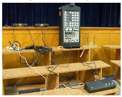
Inside the wireless mic case is an AC power strip and an AC extension cord (if needed). Use the AC power strip to plug in EVERYTHING, since that will reduce the chances of AC hum. There is also an AC "Y" cable that you can use for the (bulky) two power supplies from the wireless receivers.
