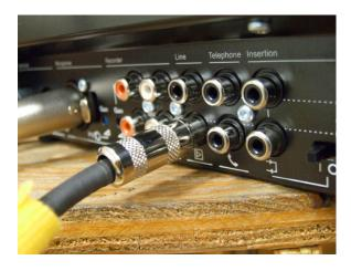
Connect the RCA cable from the back of the Conference Control Unit (marked AMP on the bottom) to the front of the Fender amplifier, marked <sup>1</sup>/<sub>4</sub>-inch **LINE** input on MIC 1.
