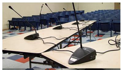
Connect each Unit to the next one in a daisy chain. Start at the far end of one table (away from the apex), and then connect the cable from each Unit to the one next to it.
