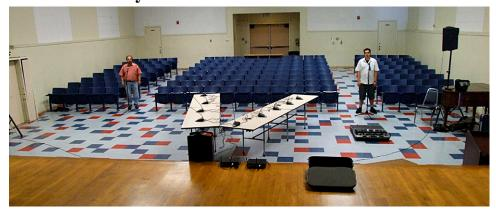
Two tables in a wide V (wider spread than shown). Note that the two speakers on stands are located on either side of the room, just forward of the tables, so that the speakers do not project audio directly into the mics of the board members.
