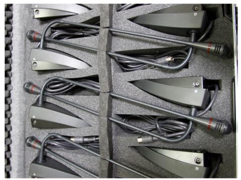
Note how the Delegate Units are packed in the suitcases. The gooseneck mics are held in place by the foam slots.
