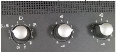
The knob on the left determines the control that the Chairman Unit has over the other Delegates. The setting shown means that only two Delegate Units can have their mics open at once, and will turn off after 30 seconds of in-activity. You could set this for one, two, three, or four mics at a time.
