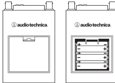
**Battery Selection** Each ATW-R1820 dual-channel receiver uses six 1.5V AA batteries, not included. Alkaline type is recommended. Always replace all batteries. Make certain the receiver power is Off before replacing batteries. **Note: The ATW-R1820 receiver also functions without batteries if connected to an external power supply (12V DC source, 500 mA nominal current, not included).**
