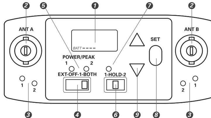
**LCD 1** Liquid Crystal Display shows battery status and frequency settings. (Use the Dual-channel Control Switch (6) to select frequencies for Receiver Channel 1 and Receiver Channel 2; in Hold position, only Receiver Channel 1 frequency appears in LCD.) Battery meter is only active when Dual-channel Control Switch is in the Hold position.
