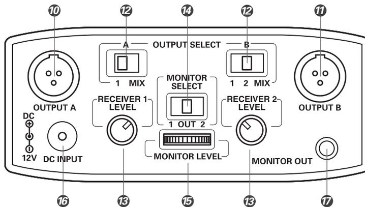
Balanced Audio Output Jack: TA3M-type connector. Pin 1: ground (shield); Pin 2: "audio +"; Pin 3: "audio -". Use the included TA3M to XLRM interface cable to connect the receiver output to a balanced microphone-level input on a camera, mixer or integrated amplifier. **10 Output A**
