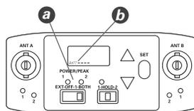
After the batteries are installed, turn the power on by moving the Power Switch to either the 1 or Both position. The small red power-on LED(s) (see *a at left*) should light (red light at 1 if Power Switch is in position 1; red light at 1 and 2 if Power Switch is in Both position) and the LCD window should come on. If this does not happen, the batteries are installed incorrectly or they are depleted.
