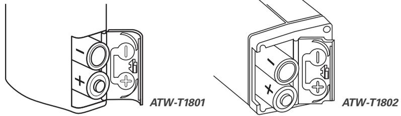
**Battery Selection** Each transmitter uses two 1.5V AA batteries, not included. Alkaline type is recommended. Always replace both batteries. Make certain the transmitter power is Off before replacing batteries.
