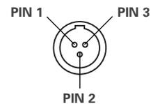
Balanced Audio Output Jack: TA3M-type connector. Pin 1: ground (shield); Pin 2: "audio +"; Pin 3: "audio -". Use the included TA3M to XLRM interface cable to connect the receiver output to a balanced microphone-level input on a camera, mixer or integrated amplifier. **11 Output B**
