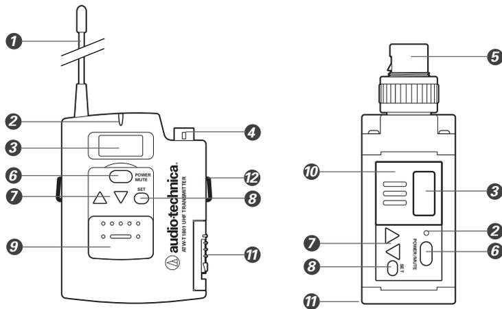
The ATW-T1801 UniPak™ body-pack transmitter includes a field-replaceable flexible antenna. For best results, allow the antenna to hang freely and full length from the bottom of the transmitter. If the received signal is marginal, experiment with different transmitter positions or try repositioning the receiver. Since the transmitter antenna simply screws in, check to make certain it is snugly attached (finger-tight). **Do not change the length of the transmitting antenna.**
