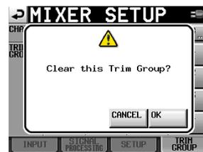
Touch the **OK** button or press the **DATA** dial to clear the group. Doing this clears the group setting from the slaves (channels with blue buttons) at the same time.
